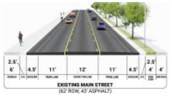
Existing Main Street Cross Section
