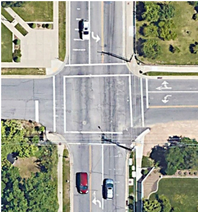
Porter Lane (400 South) & Main Street - This intersection is currently stop-controlled in the eastbound and westbound direction and flows freely in the southbound and
